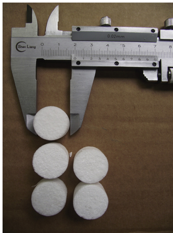
Fig. 1. Optical image of PLLA scaffold prepared by supercritical phase inversion process.
